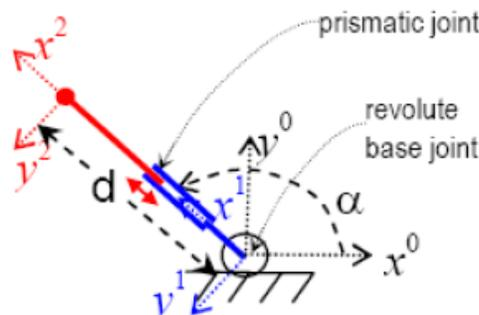
**A revolute joint** provides purely rotation around z-axis of the coordinate-frame of the previous link with the joint displacement. In the Figure you see a revolute and a prismatic joint on a planar kinematics system.  $\alpha$  Represents the revolute displacement of the base-joint, and  $d$  is the displacement joint.
