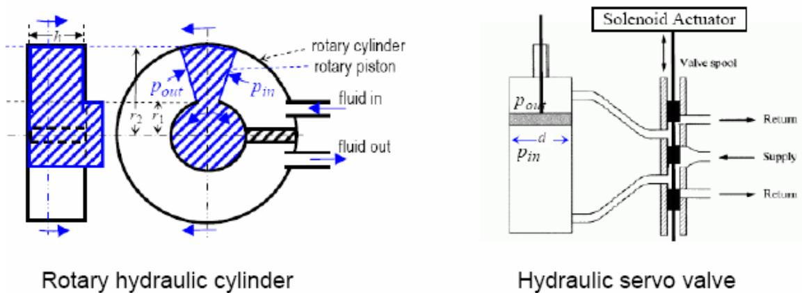
In heavy industry robotic application, pressures up to  $100 \text{ kg/cm}^2$  and up to  $50 \text{ cm}^2$  piston areas are possible, giving up to 5000 kg of force (50000 Newton). In rotary cylinders, the total output torque is obtained by the integral of the force on torque arm.
