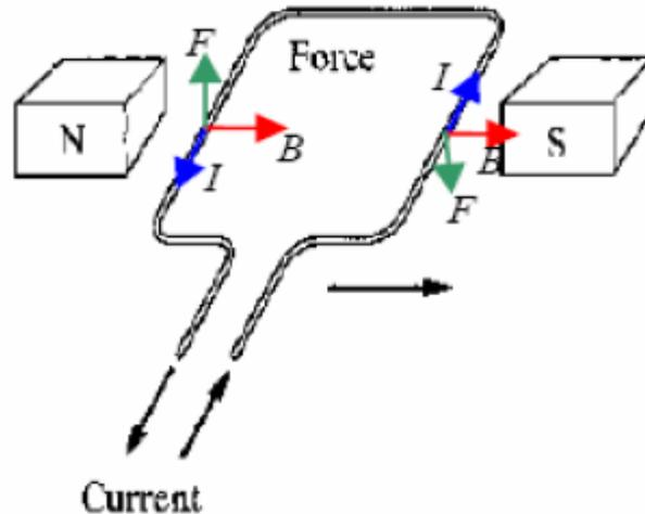
A current passing through a wire in a magnetic field produces a force.
