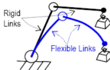
**A joint** provides movement of two contiguous links with respect to each others coordinate frames.
