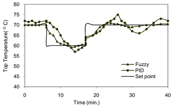
Figure(16) Comparison between fuzzy controller and PID controller of distillation temperature for step change in setpoint.
