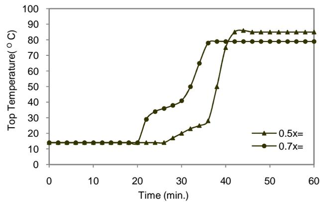
Figure(7) Open loop top temperature response at various mole fraction of MEK.
