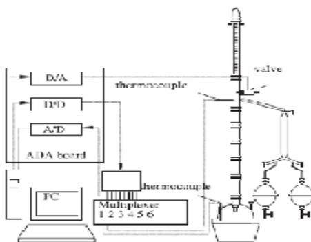
Figure(3) Schematic Diagram of the batch Distillation column.
