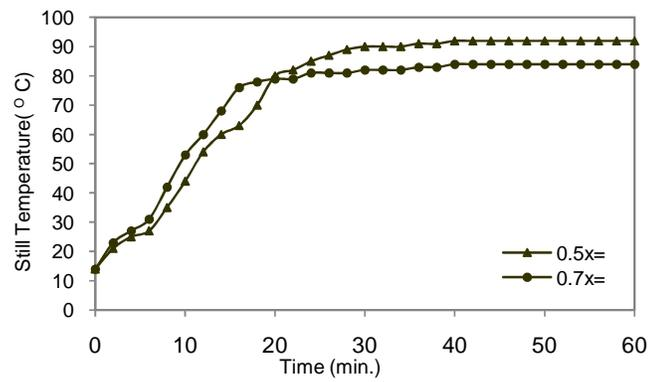
Figure(9) Open loop still temperature response at various mole fraction of MEK.
